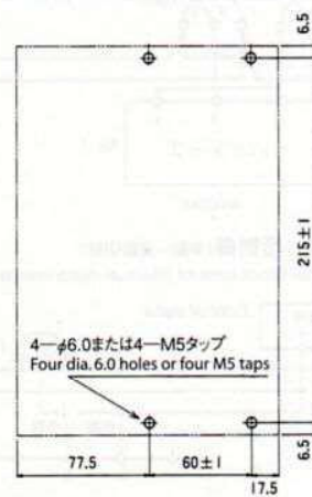
取付穴加工図 Mounting hole drilling diagram
